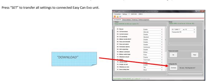
Connect a new Easy Can Evo unit to the PRG007 interface. Wait till the connection is done and press "DOWNLOAD" and "SET" command. Wait till progress bar have finished. Now the new Easy Can Evo unit is programmed and can be disconnected.
