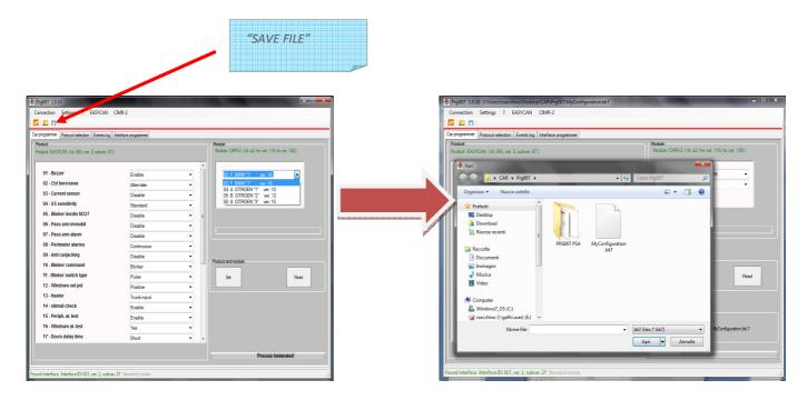
To set up more Easy Can Evo units with the stored setting file it will be possible to upload with "OPEN FILE". Point out the stored file "e.g. My Configuration". On "CAR PROGRAMMER" screen will appear a new windows "CONFIGURATION FILE" with "DOWNLOAD" command . Press "DOWNLOAD" and wait till process is terminated (see tool bar on the bottom right)
