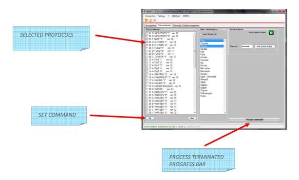
Now it is possible to "Block" the protocol selection under password (psw. must be formed by 6 numbers)
